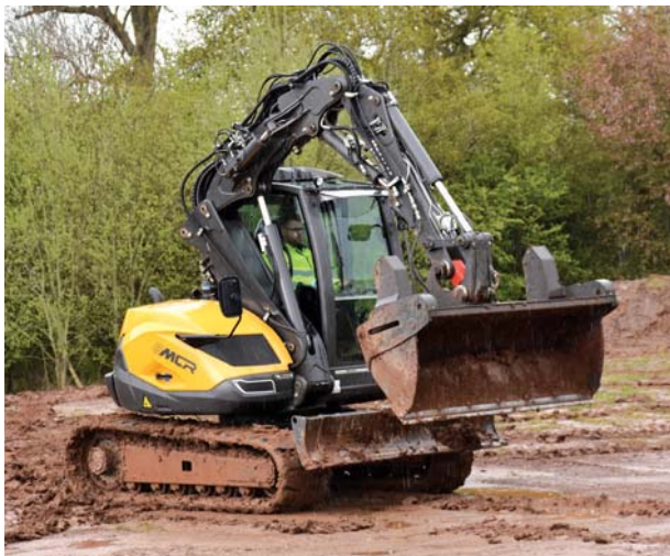
Crawler skid excavators are designed to have the compactness of a mini-excavator and the speed of a CTL to bring more versatility, range of motion and efficiency to a variety of applications. All photos by Mecalac
