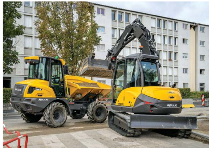
From a single position, a crawler skid excavator maintains space management, increasing productivity by letting contractors dig, break or perform a number of functions within a compact 9-foot (2.7-meter) radius.
