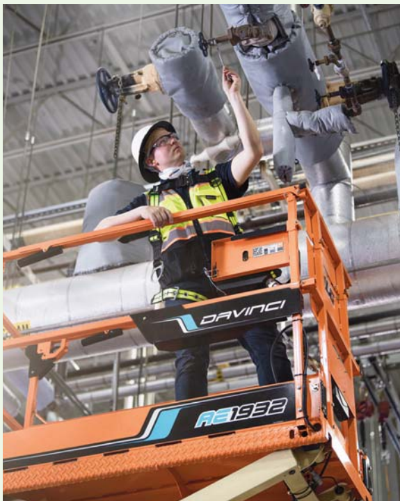
The DaVinci scissor lift system is engineered to recover energy as the platform descends, sending it back to the battery to help maximize use between charges.
