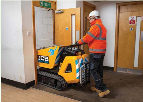
JCB's lithium-ion battery pack powers the machine for a typical full day work shift. With the smart step feature, stepping off the machine isolates power to the tracks while still allowing use of the hydraulics. Photo by United Rentals
