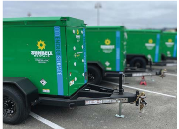
Power to recharge multiple electric machines is contained with Moxion’s tow-behind MP-75/600, giving battery electric equipment users the ability to repower at the jobsite without connecting to the grid.
