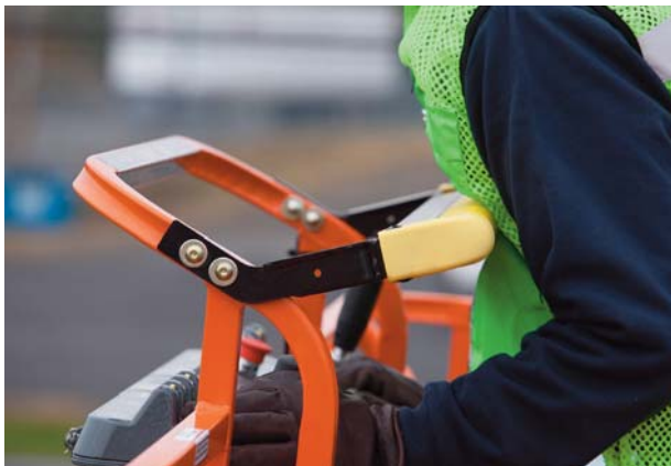
JLG SkyGuard technology offers enhanced control panel protection to reduce the risk of being caught-between hazards on the job.
