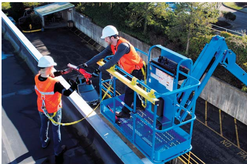
Fall Arrest Bar was designed to allow an individual to exit a Genie boom at height while being attached to a single lanyard anchor point that traverses the entire width of the platform, allowing the individual to move freely around outside the platform without the need to move the lanyard from anchor point to anchor point. Photo by Genie
