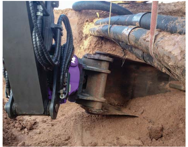
Mazio tilt-rotators not only rotate 360°, but they also tilt side-to-side by up to 55°. Photo by Mazio
