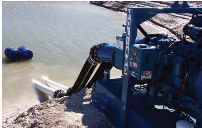
Left: Performing a bypass at a major lift station in South Florida that pushes 7000 GPM at 130 TDH, Holland uses 8-inch and 12-inch suction lift pumps.
